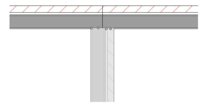
3. With the **Select Objects** \( \strace \) tool still active, click and drag the edit handles to snap the layers of one wall to the desired layers of the other.
