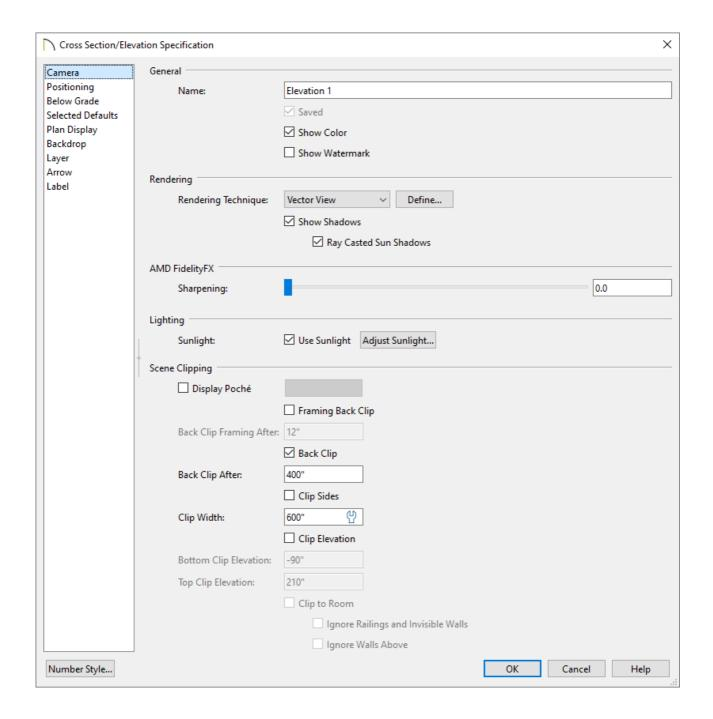
Check **Display Poché\*** to apply a dark fill to the clipped edges of walls, floor and ceiling platforms, and roof planes in the view.
