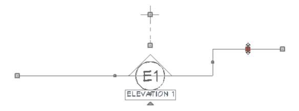
4. Click and drag the edit handle associated with the break parallel to the cutting plane to adjust the position of the step.
