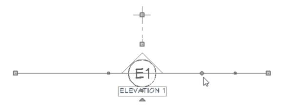
3. Click and drag the edit handle on either side of the break perpendicular to the cutting plane to create a step.
