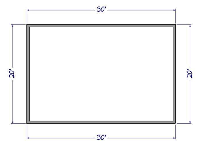
2. Using the **Select Objects** tool, select the walls that you would like to make gable walls, then click the **Open Object** determined edit button.
