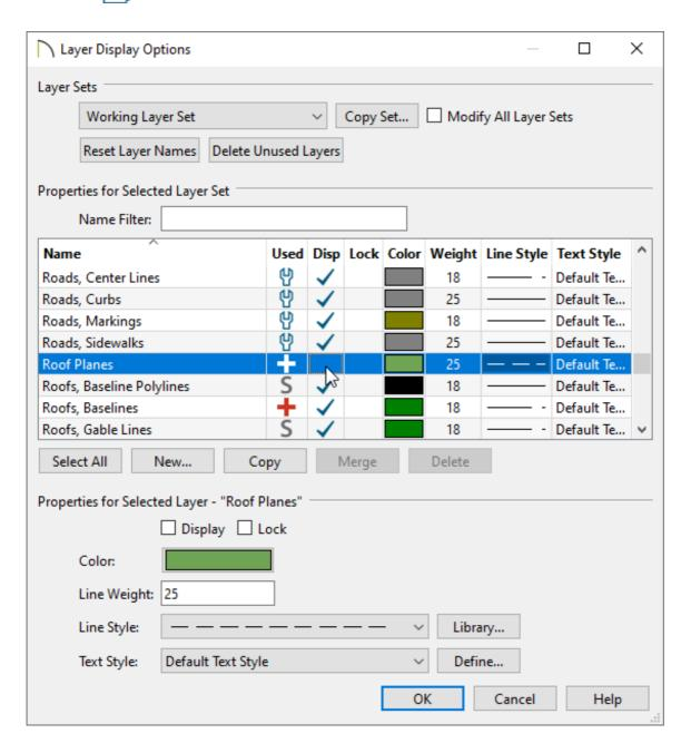
Scroll down to the "Roof Planes" layer and remove the check in the **Disp** column or from the **Display** checkbox.
