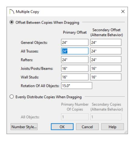
5. Hover over the main Move edit handle on the truss until you see the **Multiple Copy**to cursor display, then click and drag across the structure to create copies 24"
