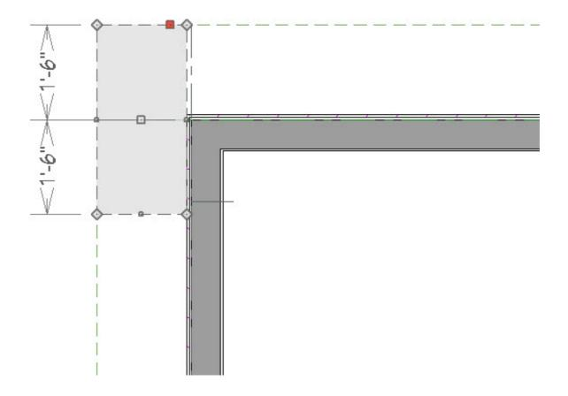
8. With the roof plane still selected, click on the corner edit handle where the ridge and outside edges meet and drag it in until it meets the corner of the wall.
