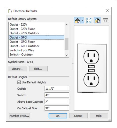
3. Next, select **Build> Electrical> GFCI Outlet**  $\P_G$ , then click in your desired location to place an outlet.
