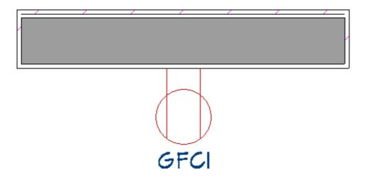
Much like the other Outlet tools, the **GFCI Outlet**  $\bigoplus$  tool can place receptacles on walls, the floor, and on the sides of cabinets and soffits.
