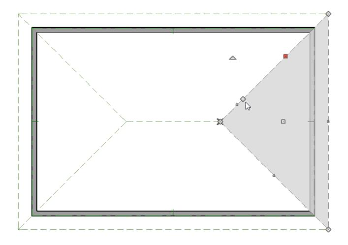
6. Click on the edit handle that displays at the peak of the roof plane and drag it down to produce a triangular-shaped opening in the roof.
