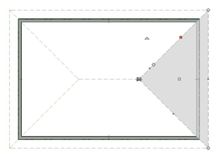
**Note:** You may want to click on the new edge to select it, click the Make Parallel edit button, then click on the wall that the roof plane is resting on to ensure the roof plane you just edited is parallel to that wall.
