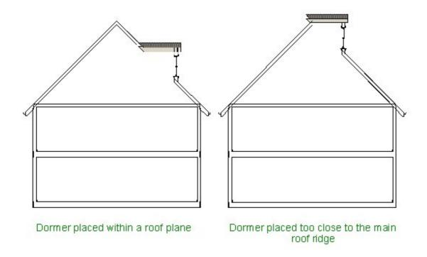
In fact, since roof planes have both a thickness and a pitch, Automatic Dormers have to
