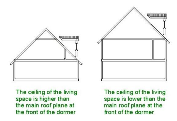
If you try to create an **Auto Dormer** at a location where the ceiling of the living space is too low relative to the roof plane on which the dormer is being placed, one of these messages will display:
