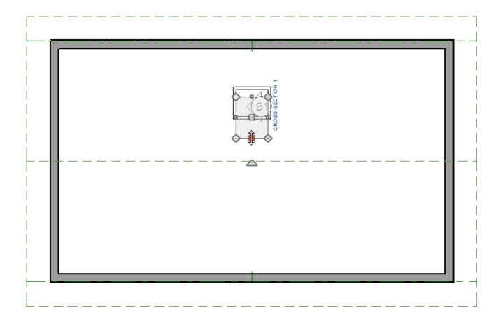
9. Continue adjusting the ceiling hole until the edge of the skylight shaft meets up with the CAD line.
