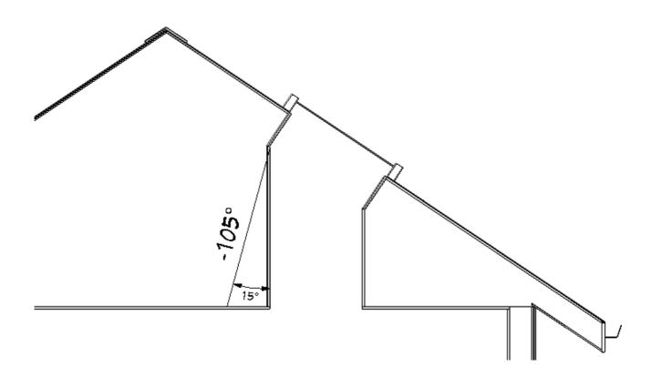
• If a specific angle is needed, you can type it in the **Line Specification** dialog.
