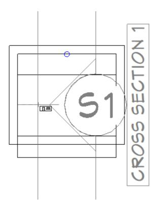
6. In the section view, select **CAD> Lines> Draw Line** / from the menu, then click and drag a line representing the desired angle of the skylight well.
