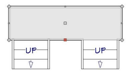
With the landing edge selected, click the Add Break – edit button, then click once between the two stair sections to break the landing's edge into two separate segments.
