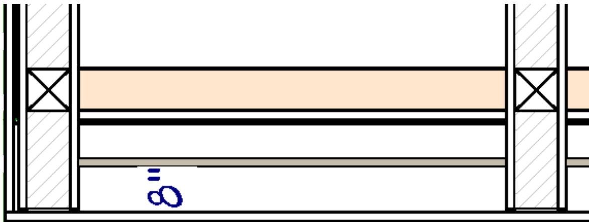
7. Use the **Multiple Copy**
