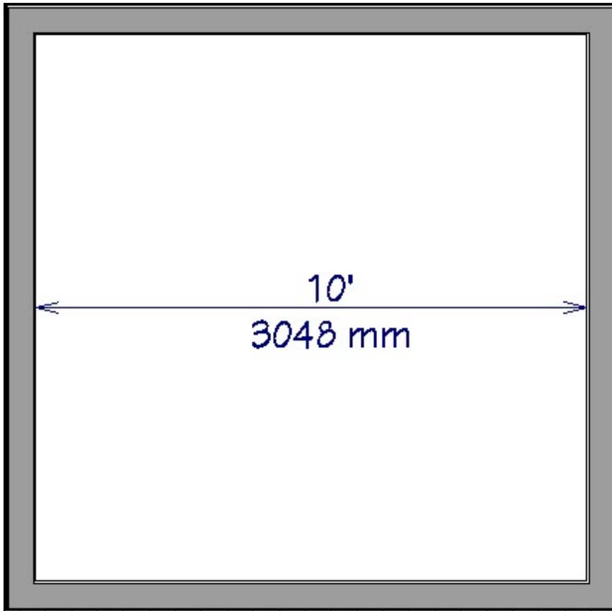
**Note:** Settings (including the Secondary Format) specified for the edited dimension line will be used when using the Add Segment edit handle.
