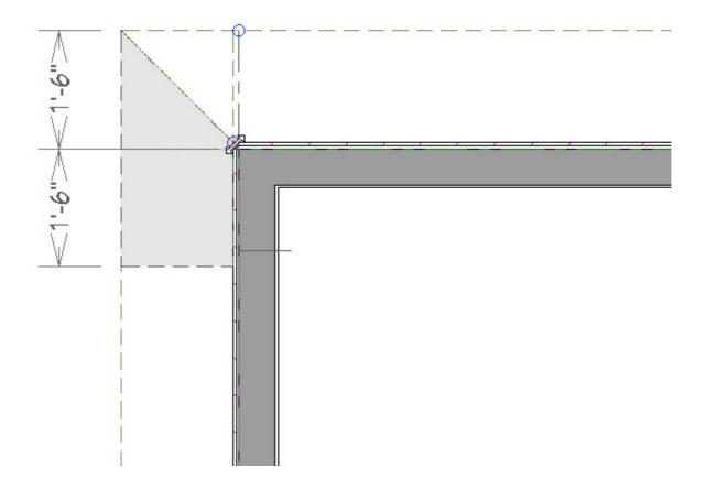
9. Repeat steps 2 through 8 on the other side of the wall to create a pair of returns, or extend this roof plane to create a full return.
