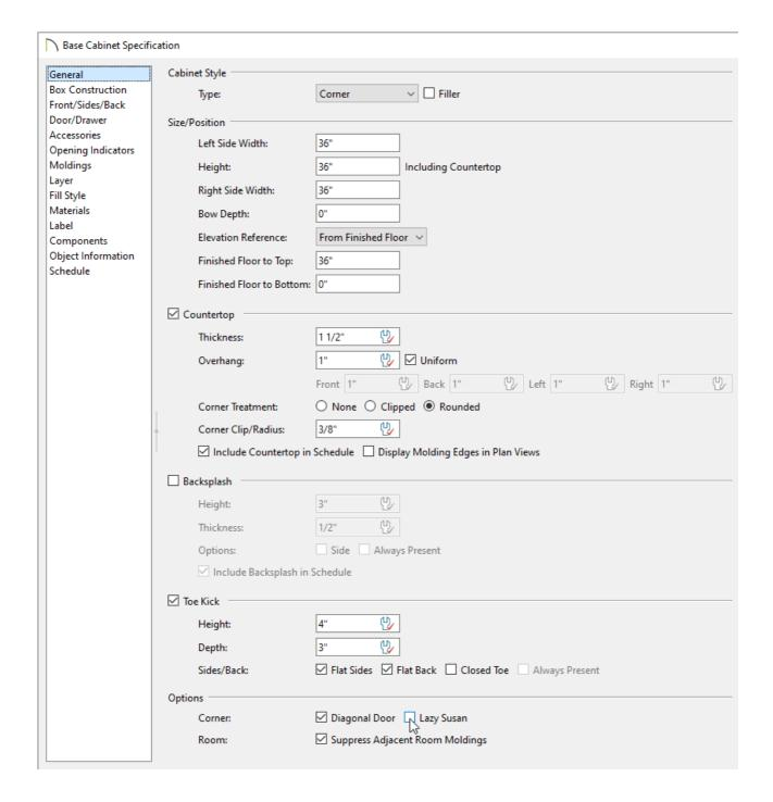
Uncheck **Diagonal Door** if you want to replace the diagonal door with double doors at right angles. This option is checked by default in the Cabinet Defaults.
