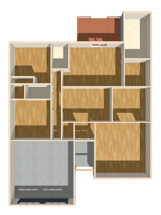
8. Additional modifications can now be made to the generated walls, doors, and rooms. You can also add additional room boxes at anytime, then perform step 6 again to generate additional walls, doors, and rooms in the plan.
