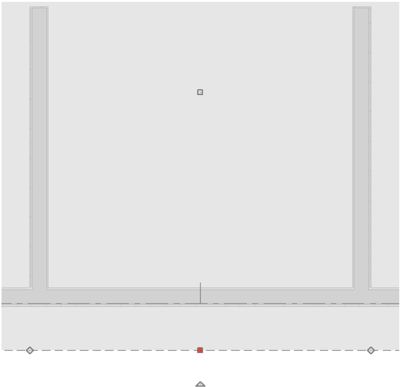
3. With the breaks placed, adjust the roof plane so it no longer covers the dormer walls. The roof plane should be snapped to the outside of the wall's exterior layer - in this case, the siding layer.
