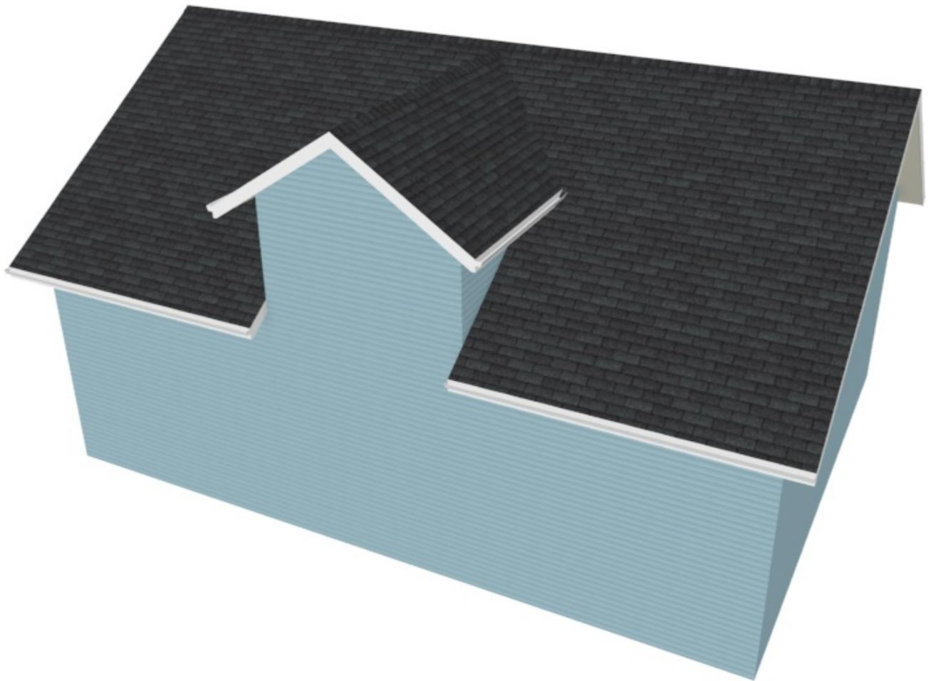
**Note:** It may be necessary to shorten or extend the length of the dormer walls depending on the pitch of the roof and how the ceiling is defined in this area.
