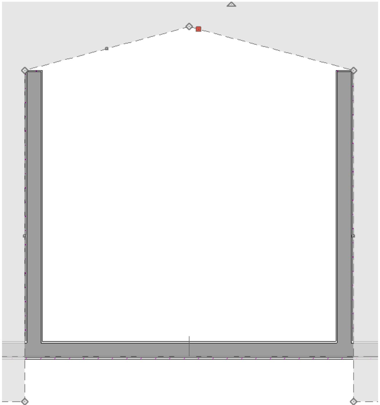
7. Next, select **Build> Roof> Roof Plane**
