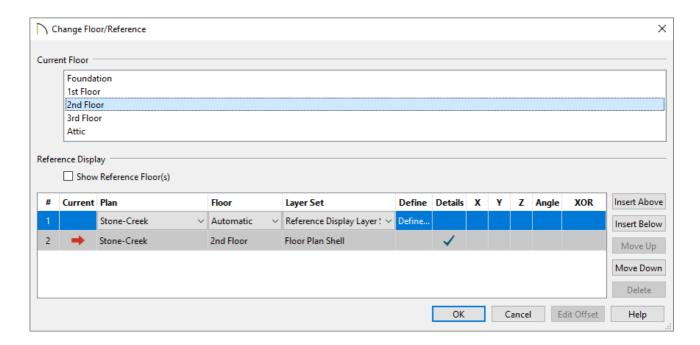
The Current Floor section will display all of the floor levels in the plan, with the currently active floor highlighted.
