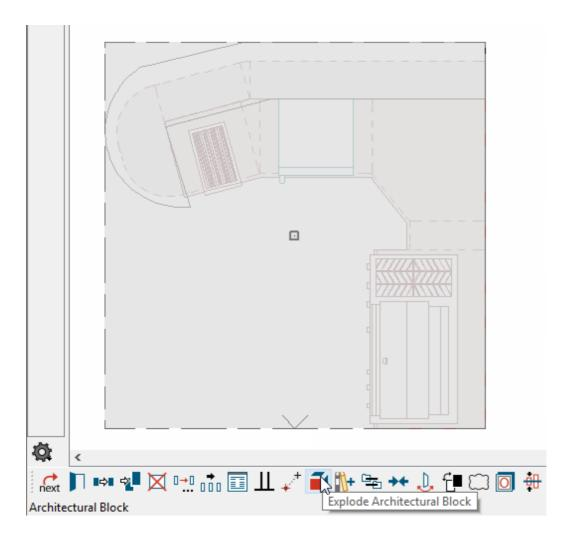
Explode Architectural Block changes the architectural block from a single, unmodifiable unit to a group of individual objects which can be selected independently.
