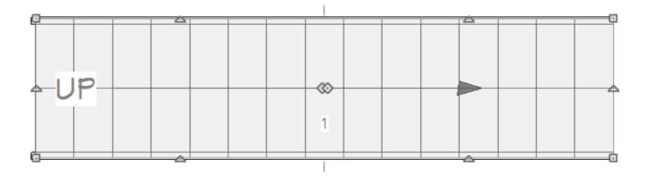
• The square handles that display at each corner of the staircase are the flare handles.
