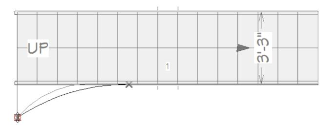
• Use the side and center edit handles closest to the flare to adjust its curve so that it closely matches that of the CAD arc.
