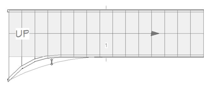
Use the dimension information that displays in the Status Bar as a reference to create symmetrical flares on both sides.
