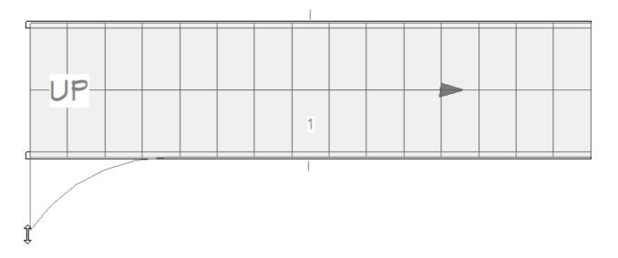
• The triangular handles that display along the long edges of the staircase are used to adjust the flare radius.
