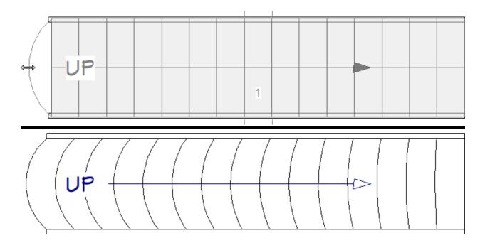
When treads are curved, all treads in the section show some degree of curvature. Treads close to the curved end have a greater curve than those at the opposite end, but both ends can be curved.
