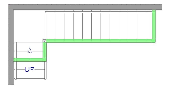
**Note:** The direction the wall is drawn will dictate how the wall is generated; if you draw the wall snapping to the edge of the Stairs, but the wall generates outside of the stairs rather than underneath it, reverse the direction you are drawing and the walls will generate underneath, rather than outside.
