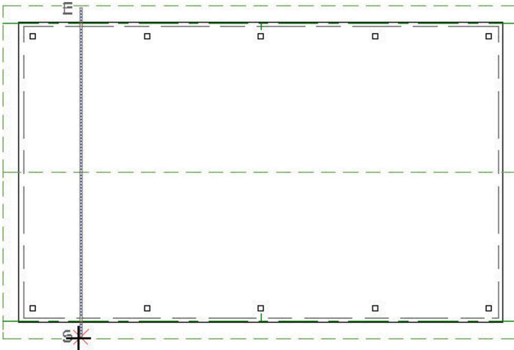
7. To move the truss over the top of the first two posts on the left side of the building, select the truss and then click on the **Center Object**
