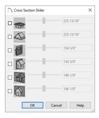
3. Check the box beside a cross section cutting plane, then either use the slider or enter a desired value using the text field.
