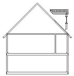
The ceiling of the living space is lower than the main roof plane at the front of the dormer
