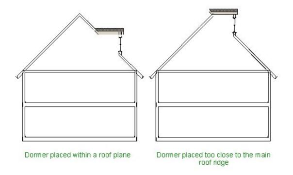
In fact, since roof planes have both a thickness and a pitch, Automatic Dormers have to be set back from the eave or ridge edges. The exact setback distance required will depend on the roof plane's depth and its pitch.
