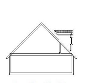
The ceiling of the living space is higher than the main roof plane at the front of the dormer
