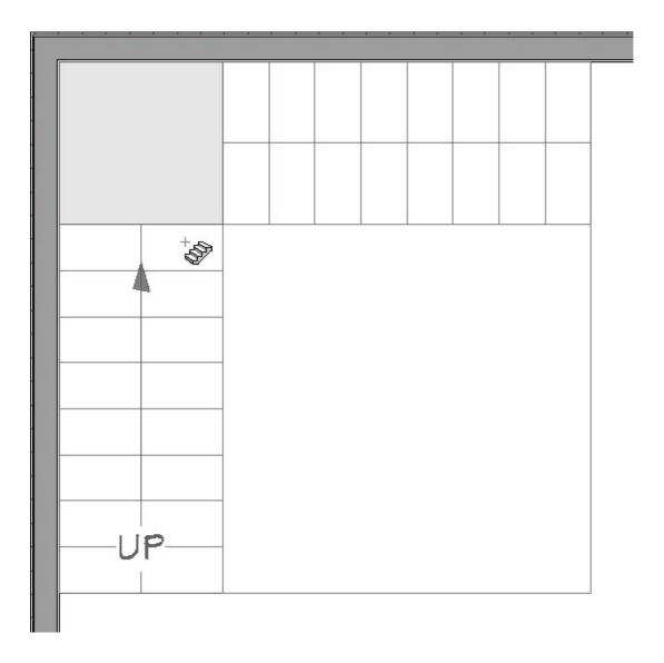
4. Click to place the stair at the desired location and the stair will be placed with a landing connecting the different stair sections.
