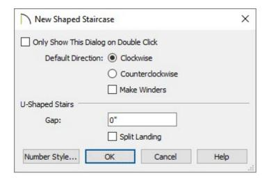
You can add winders to L-Shaped stairs, which will split the landing into two sections or create a split landing on U-Shaped stairs, which will split the landing in half by default.
