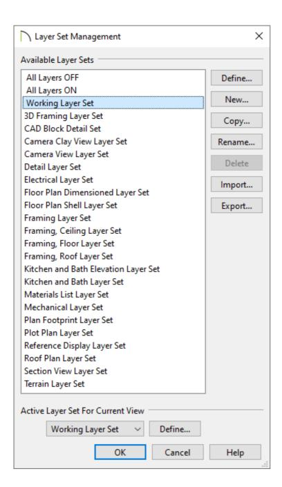
To customize layer properties for an existing Layer Set, select the name of the Layer Set to highlight it, then click **Define** to open the **Layer Display Options** dialog.
