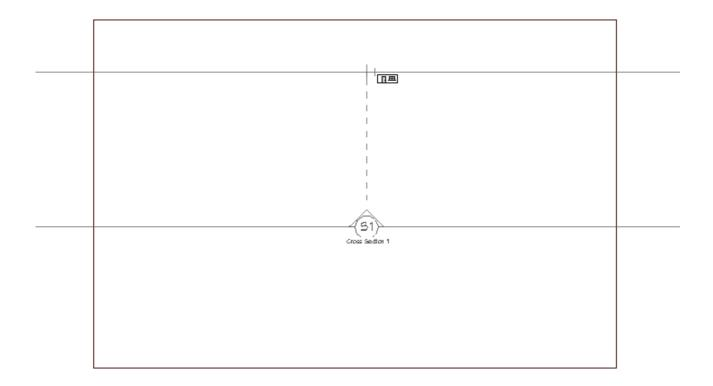
2. In the back clipped cross section view, select **CAD> Boxes> Rectangular Polyline**from the menu, then click and drag to draw a rectangle along the bottom part of the pool.
