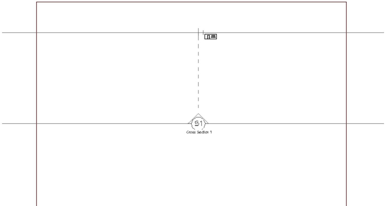
2. In the back clipped cross section view, select **CAD> Boxes> Rectangular Polyline**
