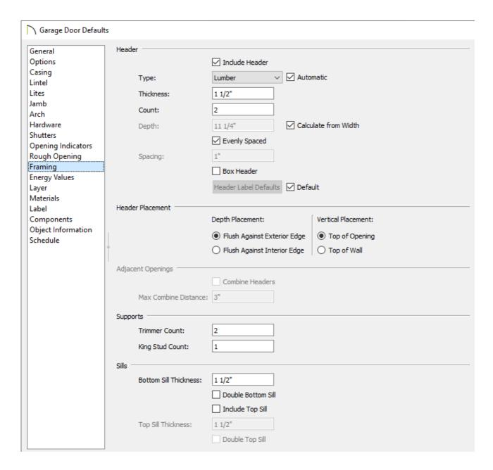
• Specify the Header Type, Thickness, Count, Depth, and Spacing.
