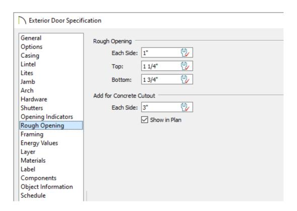
• In the **Rough Opening** section, add the **Top** value to the **Height** of the door and make a note of the total. This total is the length that the door trimmers need to be to reach from the header down through the concrete cutout to the floor.
