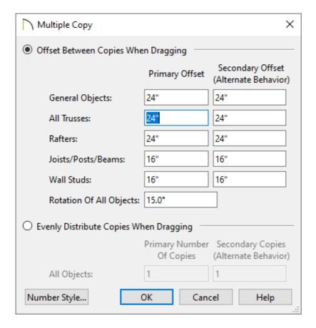
6. Hover over the main Move edit handle on the truss until you see the **Multiple Copy**trusses will be created at regular intervals. Release the mouse button to complete the command.
