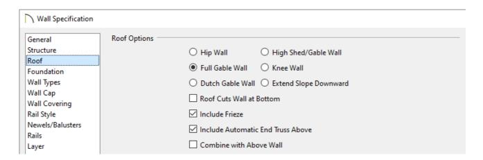
For additional information on building an automatic gable roof, visit the "Generating Automatic Hip and Gable Roofs" article linked in the Related Articles section below.
