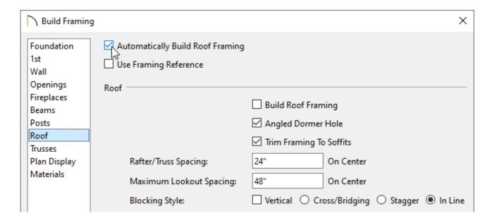
Automatic trusses, along with any other automatic framing components, such as blocking and fascia boards, will be generated.
