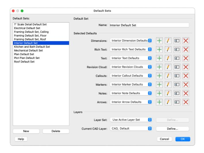
7. In the **Default Sets** dialog, either click the **Define** button to the right of **Current CAD Layer** and create a new layer for CAD objects to be drawn on when your new
