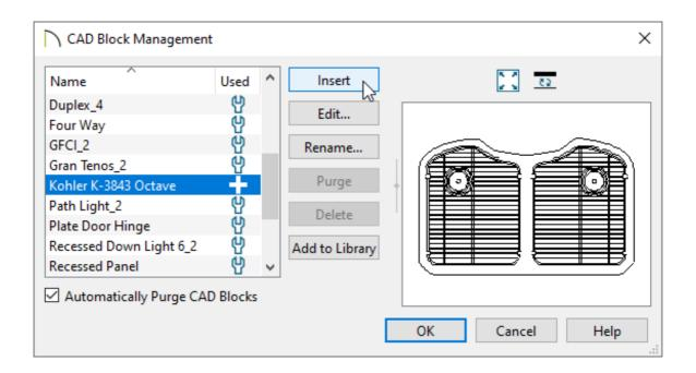
4. Click in an empty area of the plan to place the CAD block.
