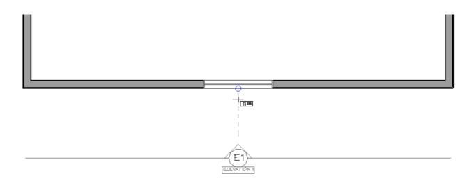
9. In the cross section/elevation view, use the **Select Objects**  $\geqslant$  tool to select the window, then use the **Move**  $\Leftrightarrow$  edit handle to butt it against one side of the wall.
