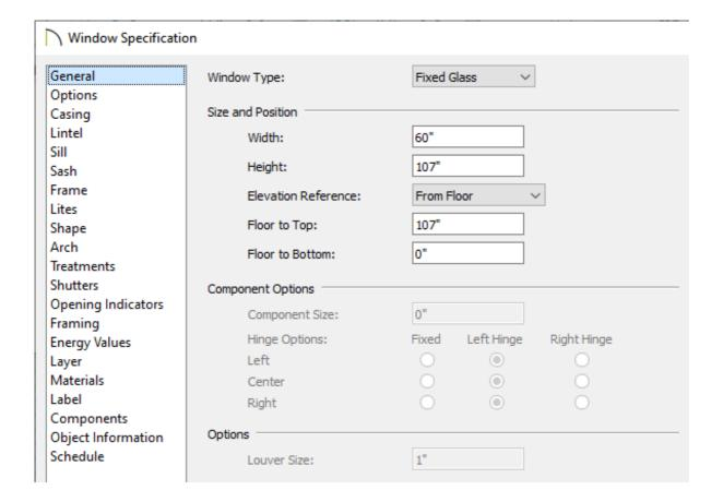
On the General panel, set the Window Type to Fixed Glass, then specify the Width, Height, and Floor to Top values to your liking.
