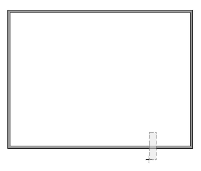
• Once the baseline has been created, move the mouse to the opposite side of the structure and click where you would like the roof plane to stop at.
