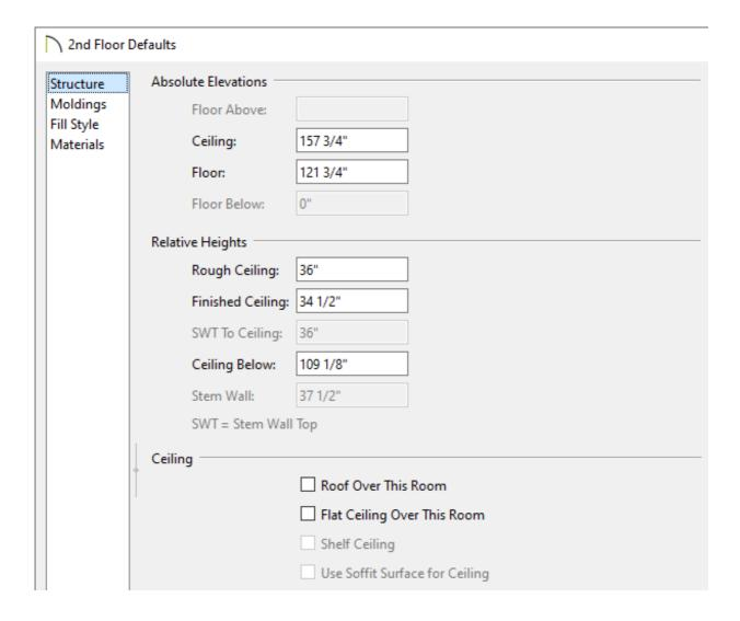
• Set the **Rough Ceiling** value to equal the height you would like your parapet walls to be.
