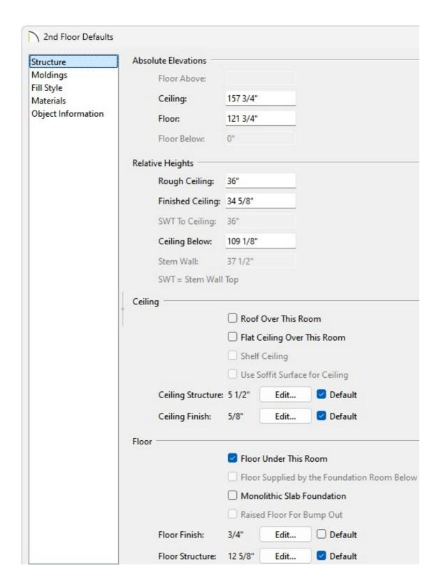
Set the Rough Ceiling value to equal the height you would like your parapet walls to be.
