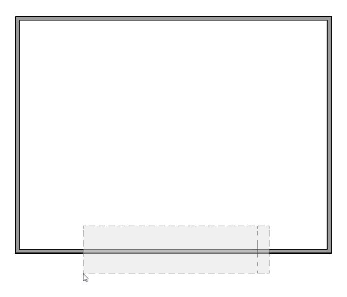
Adjust the left and right edges of the roof plane, as needed. The left edge of the roof plane will be where the arch starts, while the right edge will be where the arch stops.
