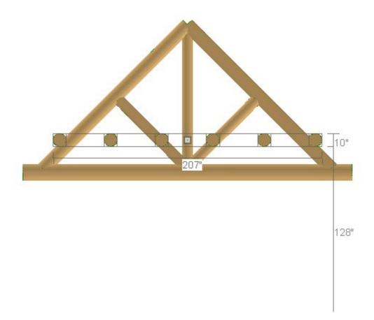
5. Use the selected set's Move edit handle to move the selected purlins straight up until they are at the height of the trusses.
