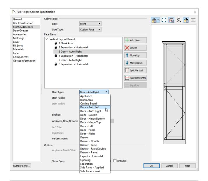
**Note:** The Auto Right and Auto Left options become double doors when a cabinet's width is greater than 24" or 600mm. The Left, Right and Double options always display as specified, regardless of the cabinet's width.
