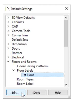
3. In the **1st Floor Defaults** dialog, specify the desired **Ceiling** height on the **STRUCTURE** panel.
