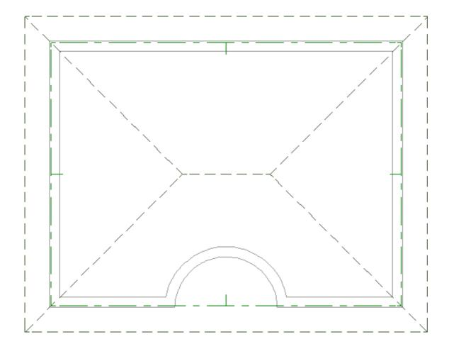
• Spanning the concave curved wall with a straight baseline, resulting in a separate roof plane.
