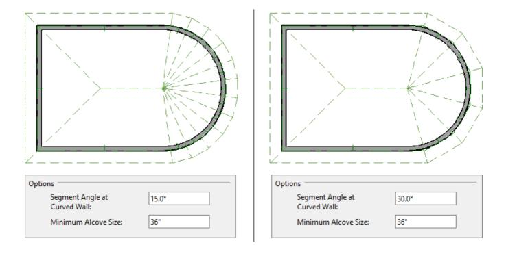
Regular roof plane sections can also generate above concave curved walls. For roof sections to generate above a concave curved wall, the sections' baselines must be longer than the **Minimum Alcove Size** value on the Roof panel of the **Build Roof** dialog.
