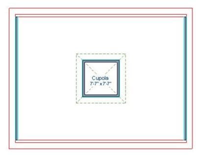
In our example, because there are two Full Gable walls set on the floor below and because the roof is set to automatically rebuild, there are automatically created attic walls to the left and right.
