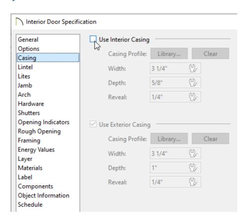
• On the Casing panel, remove the check from the **Use Interior Casing** box.
