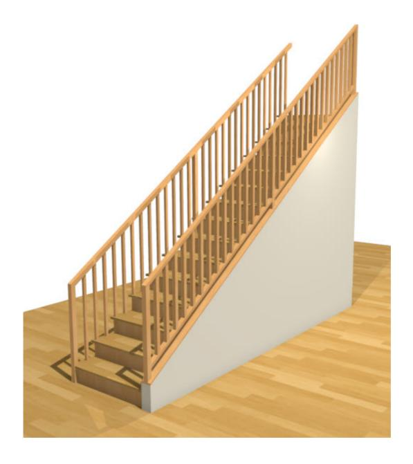
Several railing and wall variations can be created alongside stairs. For example, you may want a railing to follow the angle of the stairs, but then die into a full height wall. Please view the <u>Stair Wall Options: Partial Railing, Wall Under Stairs, Stairwell</u>
