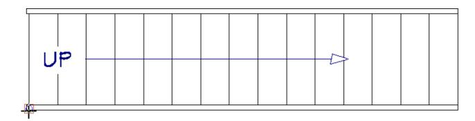
It's important that you don't create or move the railing beneath the stairs. If you're having trouble precisely placing the railing beside the stair section, navigate to Edit> Snap Settings and ensure that your Object Snaps are enabled.
