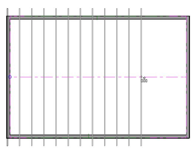
The trusses located on each end of the structure will be a full size trusses. If you wish to have end trusses instead, group select the trusses on each end, open them up to specification, check the "End Truss" and "Force Truss Rebuild" boxes, then click OK.
