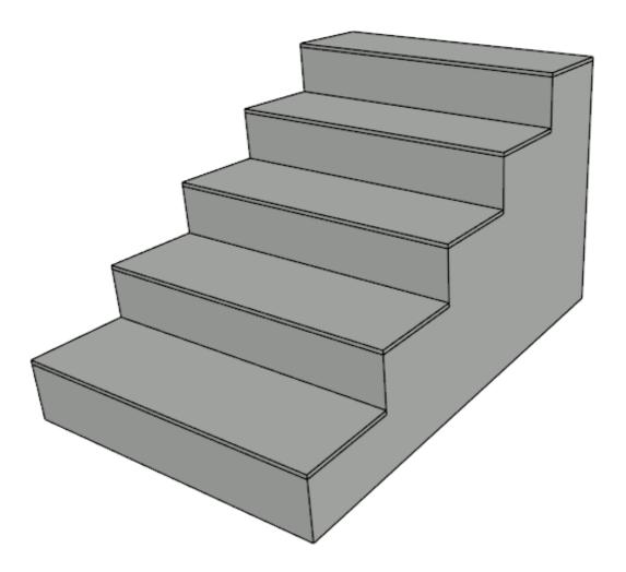
The staircase shown below is using a 1" Tread Overhang and a 1" Tread Thickness.
