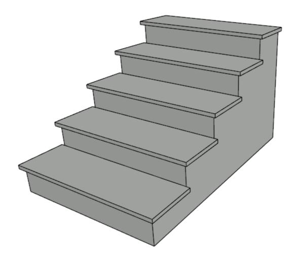
The staircase shown below was created by using Custom Stringers and setting both the Left and Right Stringer to have a 3" Extension above the tread.
